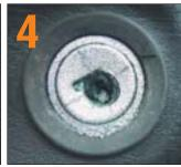
Use a pick tool to dislodge the lock bar that prevents the cylinder from turning.
