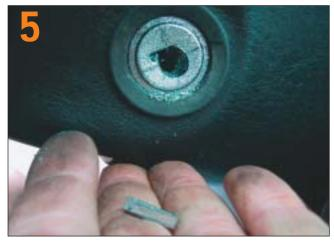
Fish the lock bar out of the cylinder.
