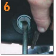
Turn the lock cylinder to the start position with a screwdriver. Note: Most of these vehicles are equipped with Ford's PATS system. You must hold the original key near the lock cylinder when the ignition is
